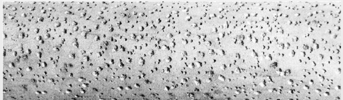
Pitting of Cr-Ni stainless steel in HCl
